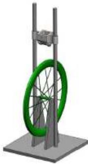
Picture 1: Vertical drop test installation
